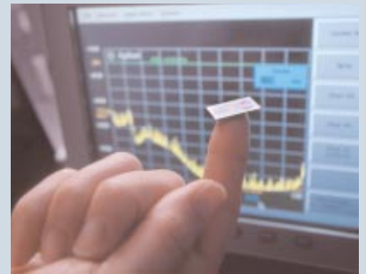
Xerox researchers have developed the Optical MEMS (Micro Electro-Mechanical Systems) switch. Photo by: John Griebsch
